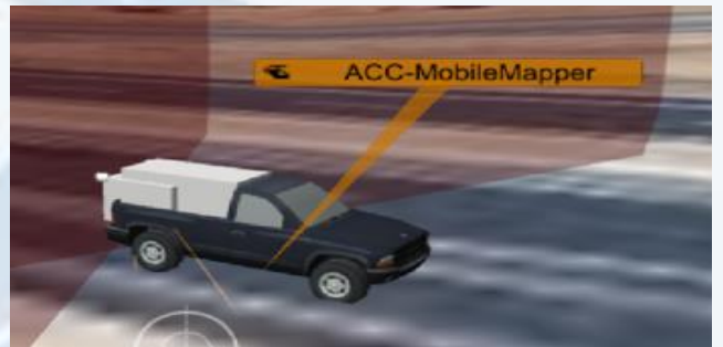
Figure 3: ACC-MobileMapper - The Acciona's MobileMapper carrying dual laser scanners analyzing the road surface.
