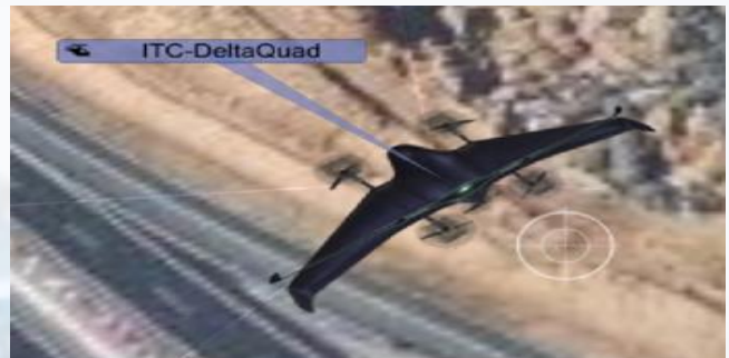
Figure 2: ITC-DeltaQuad - A hybrid drone carrying an RGB camera. The footprint of the camera is displayed in real time on ground surface
