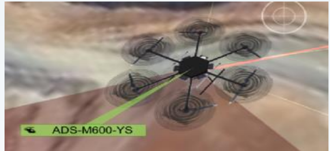
Figure 1: ADS-M600-YS - An Airbus UAV carrying a YellowScan lidar scanner.
