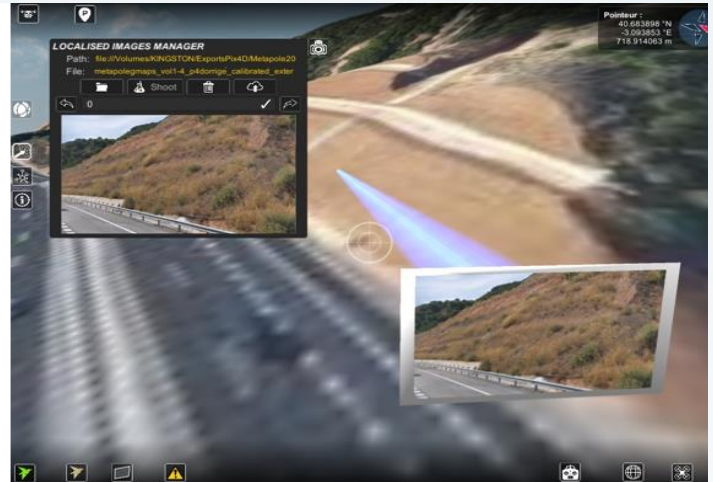
Figure 7: Presentation of the Localised Image manager and examples of a shot over the Guadalajara slope (simulation). The pictures appear "floating" in the air at the position and direction they were shot.
